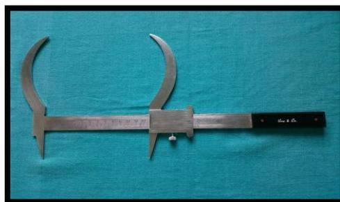
Fig-2: Sliding Calliper
