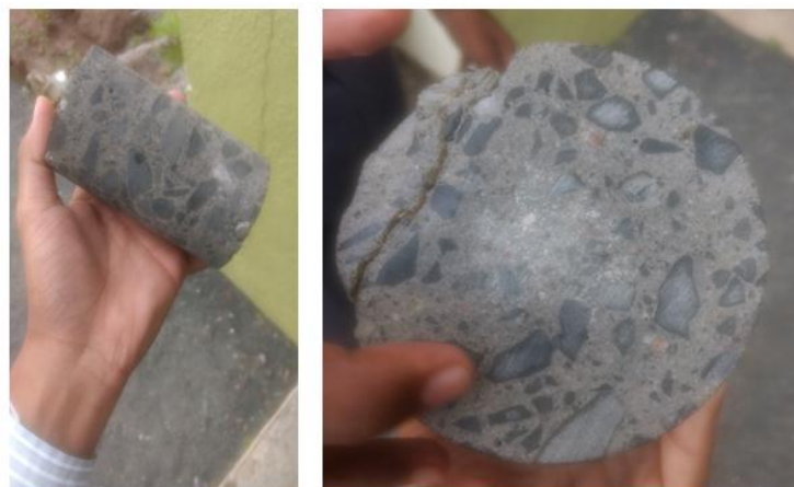
Fig-5: Cores after water absorption
