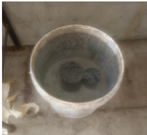
Fig-4: Cores placed in water for 24 hours
