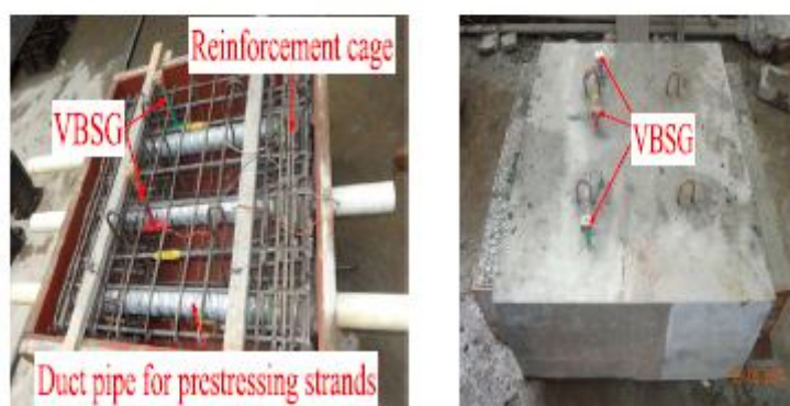
Fig-3: VBSG in slab [12].
