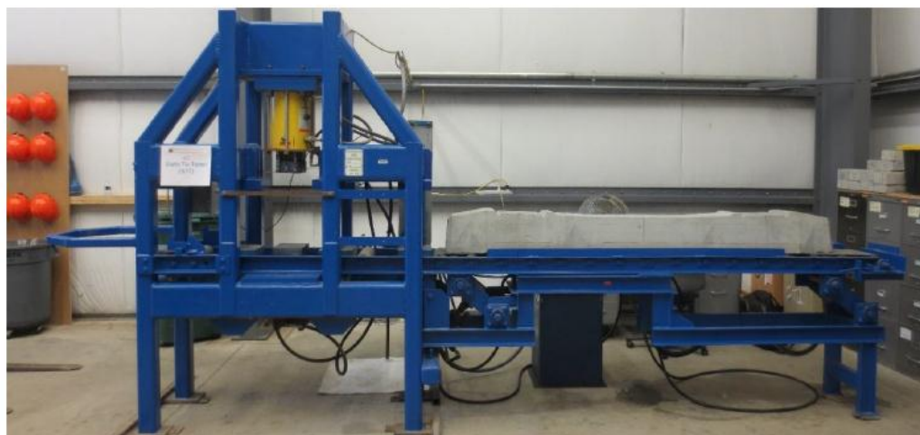
Fig-2: Static Tie Tester (STT) at UIUC used for laboratory calibration of concrete sleepers [3]
