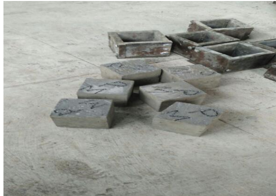
Fig-1: Casted cubes after 24 hours
