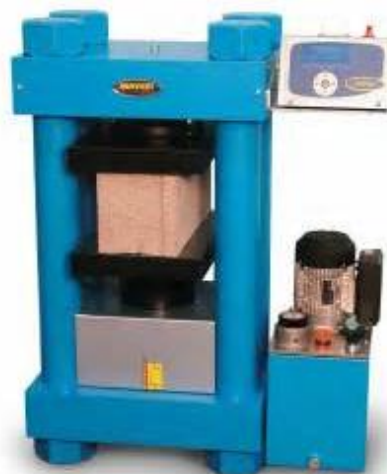
Fig-3: Compression Testing Machine
