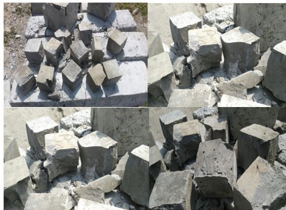
Fig-2: Casted Cubes after Compressive Strength Test
