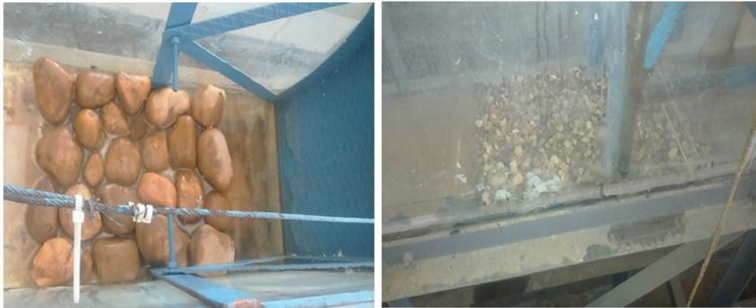
Fig-1: The gravel beds used downstream the radial gate.
