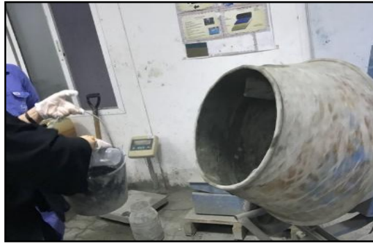
Fig-3: Mixing the quantities of materials (Source: CCE ML)
