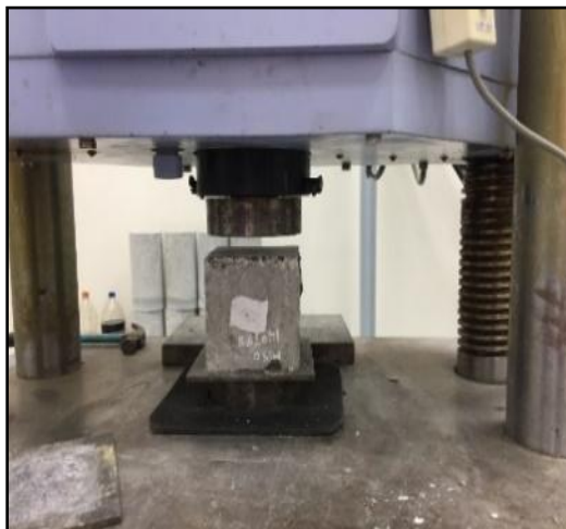
Fig-9: Compressive Strength test (Source: CCE ML)
