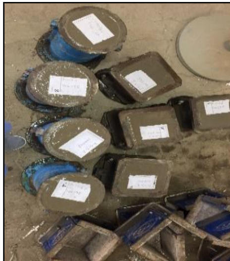
Fig-7: Casting Cubes and Cylinders of Porous concrete (Source: CCE ML)
