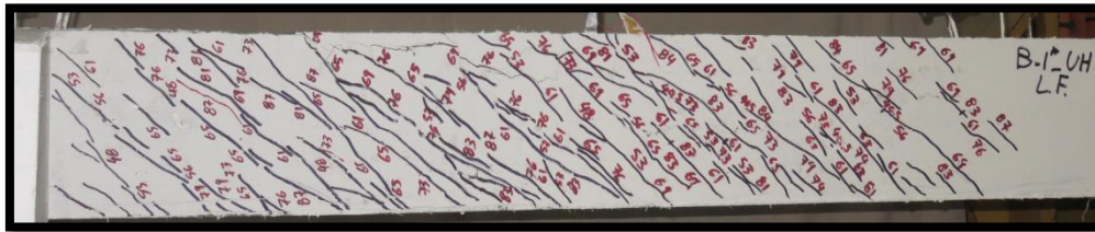
Fig-12: Crack pattern of beam B-1* -UH at failure
