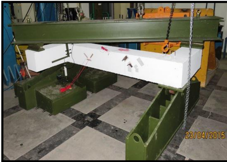
Fig-4: Loading set-up of the beams
