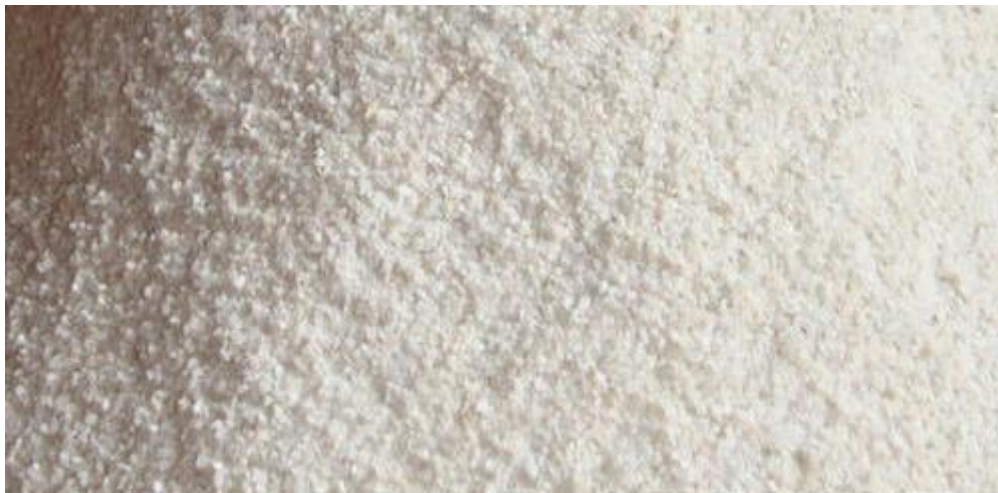
Fig-7: Picture of Marble Dust Majorly Used As Replacement of Cement in Pakistan
