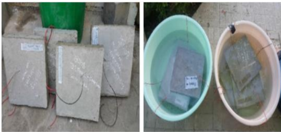
Fig-7: Slabs before & during curing
