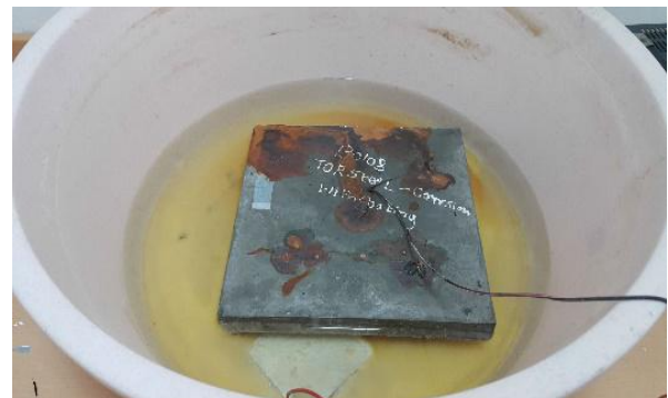
Fig-10: Corrosion in process
