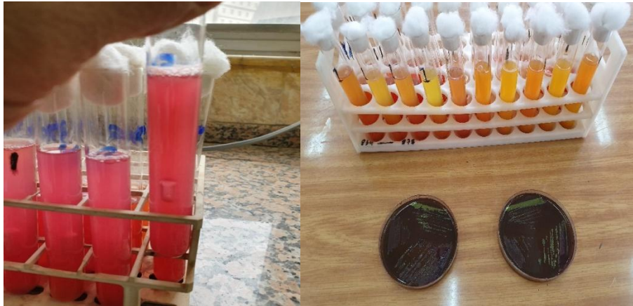
Fig-2: Show the fermentation and gas production for the positive water sample with coliforms contamination
