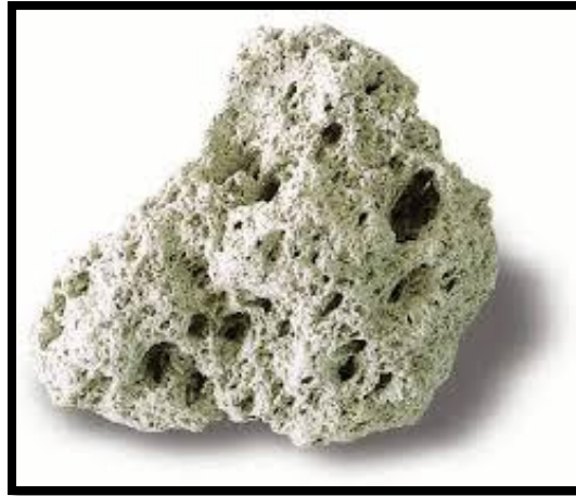
Fig-1: Surface porous on the pumice aggregate
