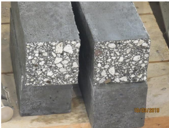
Fig-4: Sample of prism after flexural failure
