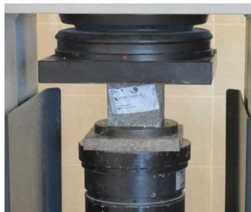
Fig-3: Compressive test of the cube
