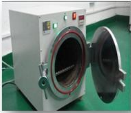
Sterilization of Diluted Agar Medium in Autoclave
