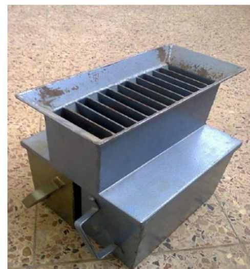
Photo: Riffle Box for quartering fine aggregates and sieves Shaker with series of sieves
