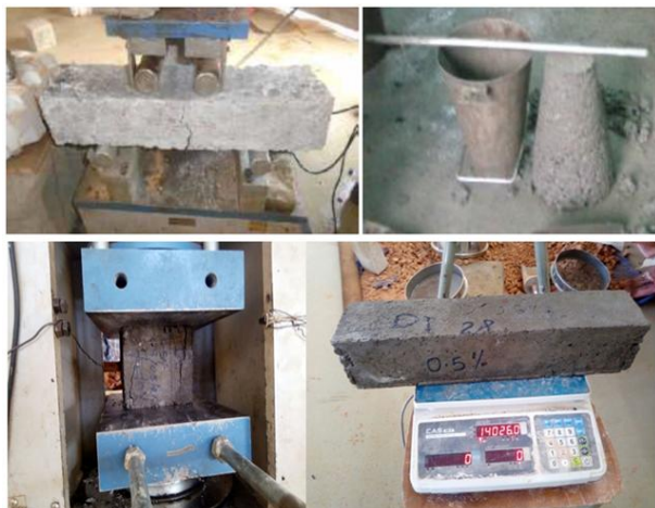
Photo: Test on hardened and fresh concrete
