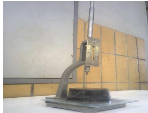
Photo: Initial and final setting time tests for cement
