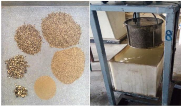
Photo: Graded fine aggregate sample and testing of absorption test
