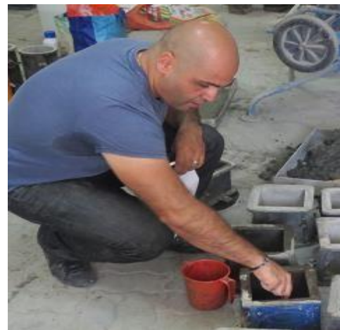
Fig-6: Application of shuttering oil to cube samples
