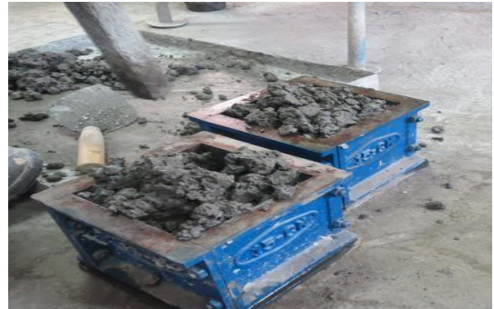
Fig-10: Transfer of concrete to cube molds
