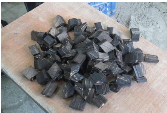
Fig-3: Tire Rubber Aggregate 20mm
