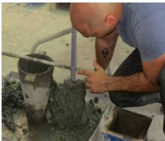
Fig-9: Measurement of slump
