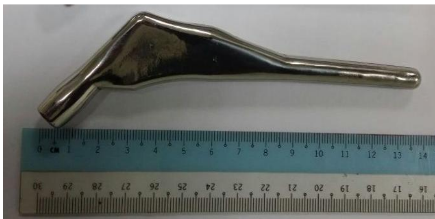
Fig-3: Sintered hip stem produced using MIM process after polishing
