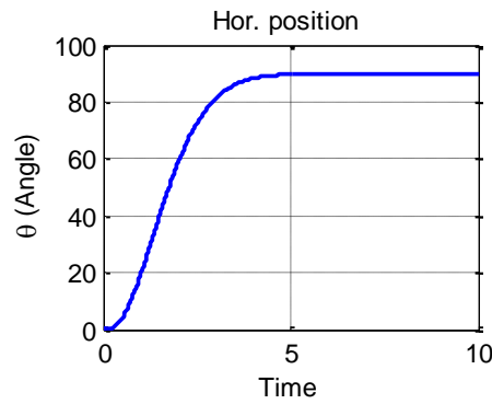
Fig-9(b): One Actuator angular displacement for 90 degrees
