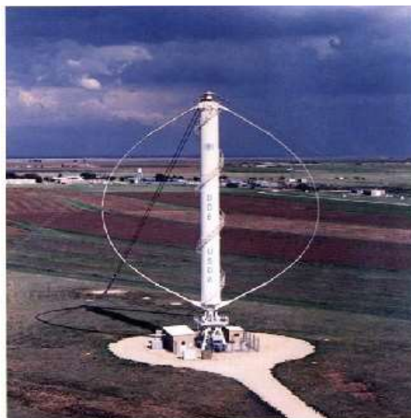
Fig-2: A Sandia turbine with 34 m diameter
