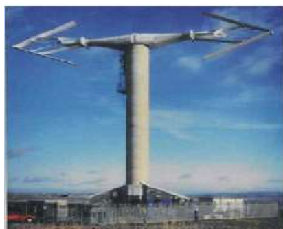
Fig-4: To the left is an H-rotor developed in the U.K. and to the right is one of the Heidelberg rotors
