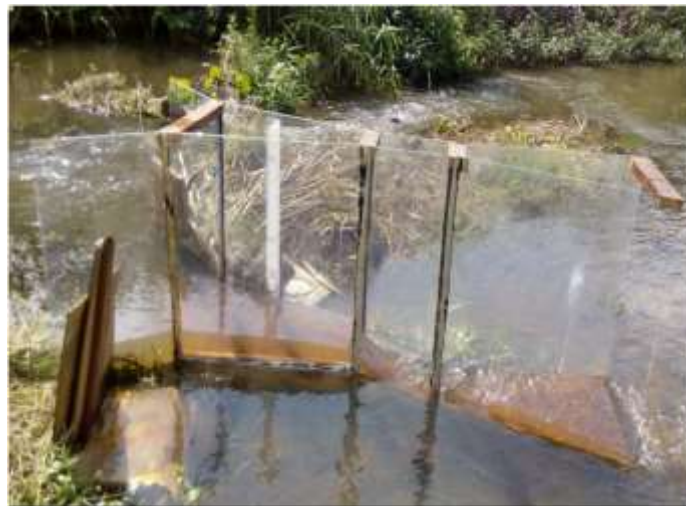
Plate2: free flow condition occurring through the parshall flume
