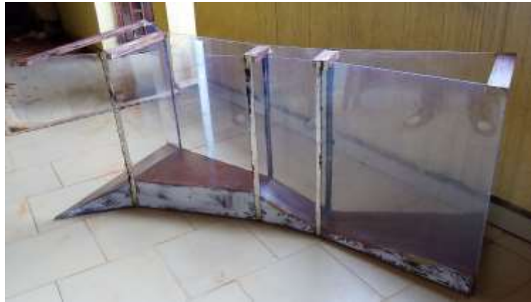
Fig-2: A fabricated parshall flume
