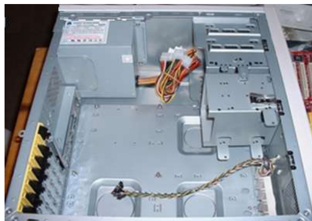
Fig-2: Chassis Case with Power Supply Unit
