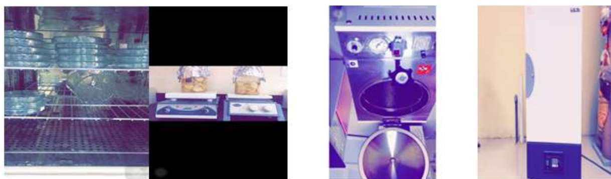
Fig.1 Laboratory equipment utilized during the project. (Hot air Oven , Heater , Autoclave and Refrigerator)
