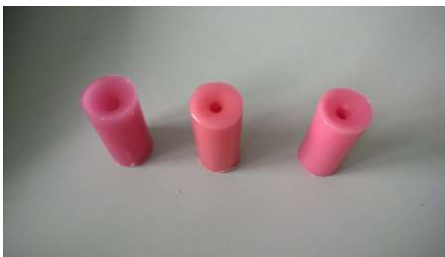
Fig-1: Visible shrinkage of waxes patterns (from left Bego, Interdent, Bredent)
