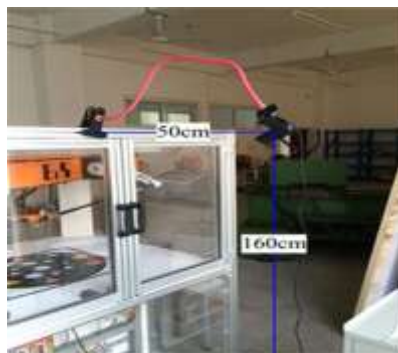
Fig-1: working platform and the installation position of the camera
