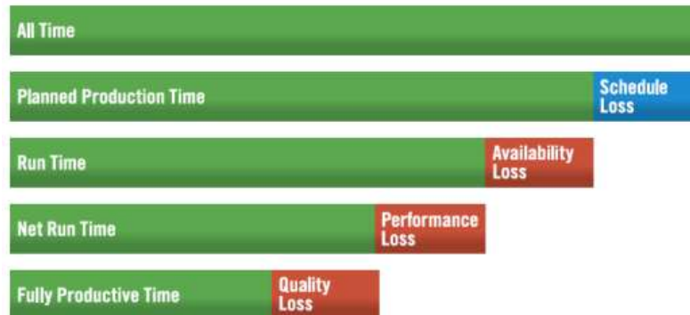
Fig-2: OEE measures the percentage of planned production time that is truly productive [16]
