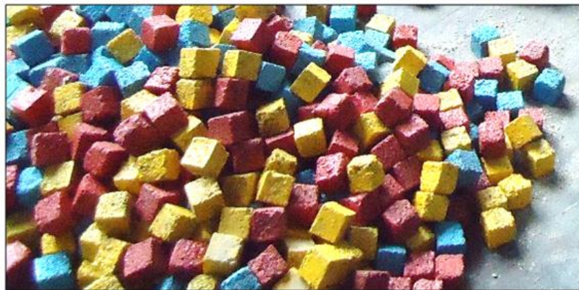
Photograph-2: Cube-shaped Concrete blocks used in the study
