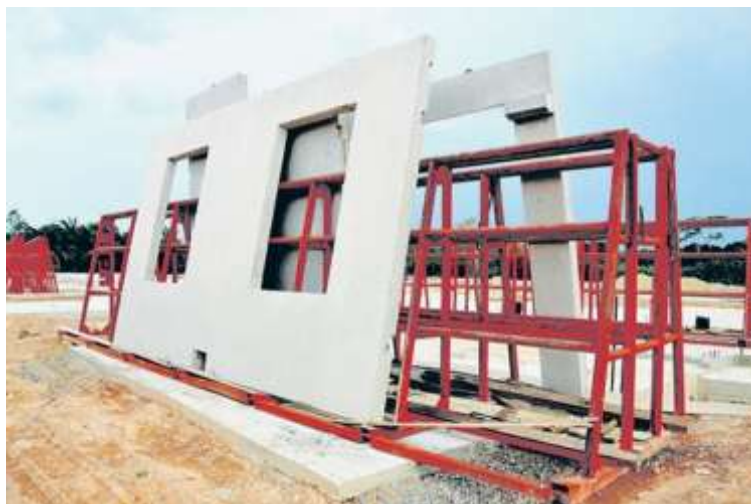
Fig-3: Wall panel in IBS system
