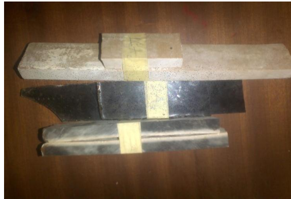
Fig 1: Specimens after Tensile Test
