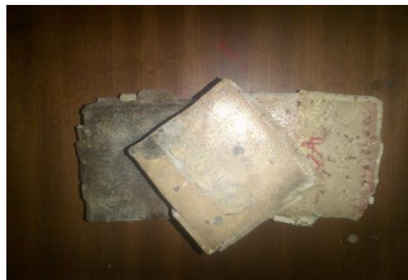
Fig-2: Specimen after Final Collapse on Compressive Test
