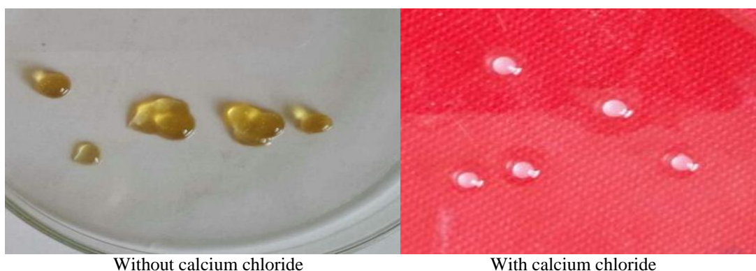
Fig-4: Effect of calcium chloride solution on beads shape and stability. Beads were heated at 70°C with and without 0.2 M calcium chloride solution for 60 min. (using a digital camera).
