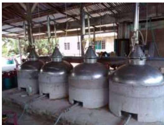
Fig-1: Hydro-distillation method of agar oil extraction
