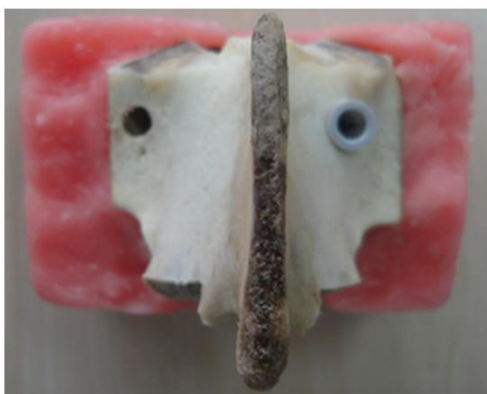
Fig-1: Wax-fixed fresh frozen calf vertebrae, a dowel is seen on the left side
