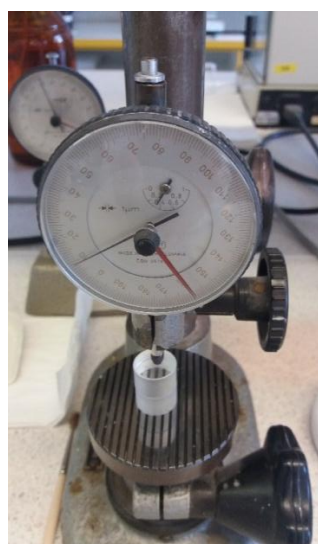
Fig-4: Samples on etching gel in under 15 kg force in mico meter
